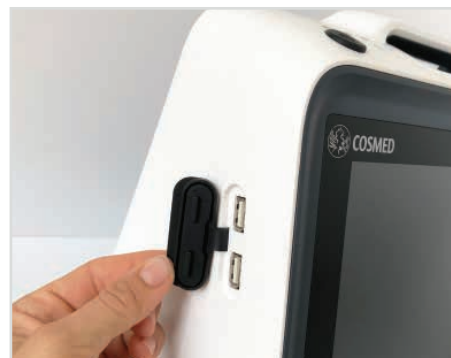
Lateral USB ports allow easy data export for efficient data management.
