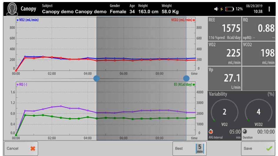
Using the Best 5 min button, the 5 continuous minutes with the lowest VO 2 and VCO 2 variability are selected and used for final results calculation.
